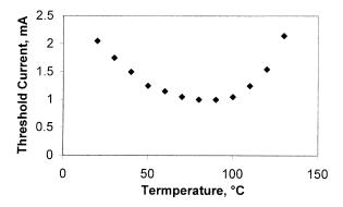
Fig. 3. Threshold current versus temperature for record high temperature device.
