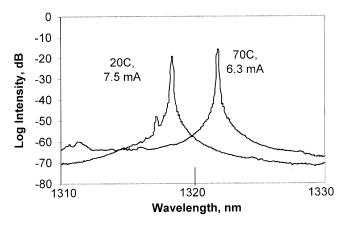
Fig. 5. Optical spectra near rollover at 20  $^{\circ}$  and 70  $^{\circ}$  C for the device of Fig. 4. Wavelength range shown is from 1310 to 1330 nm.
