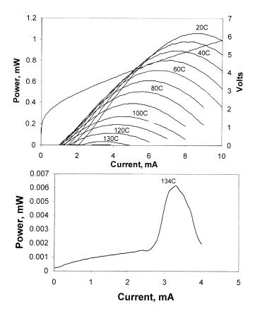
Fig. 2. The 8- $\mu$ m device with record 134 °C maximum CW operating temperature. Upper chart illustrates the *L-I-V* curves from 20 ° to 130 °C (voltage is at 20 °C). Bottom chart shows the *L-I* at the maximum CW lasing temperature of 134 °C.
