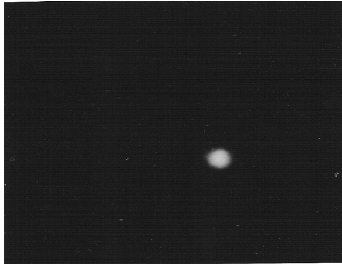
Figure 4.4.3 Photo of the laser beam spot taken at 1 m away from the output coupler of the external-cavity VCSEL shows that the laser beam is transversely single mode.
