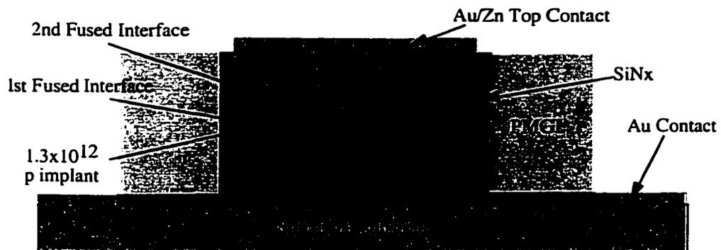
Figure 8.7 – Cross-section diagram of a second generation InGaAs-silicon APD. This device was created through RIE etching and encapsulated with dielectric layers.
