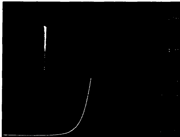
Figure 3.07. Curve tracer I-V characteristic in constant current mode showing a kink at 9mA with a magnitude of greater than 3V.
