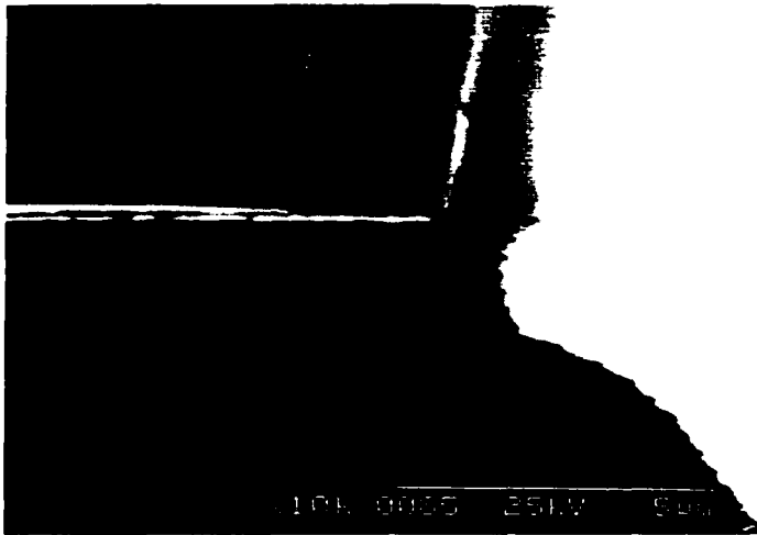
Figure 5.08 Example of undesirable sidewall profile frequently obtained after plasma-therm RIE has been opened for maintenance.
