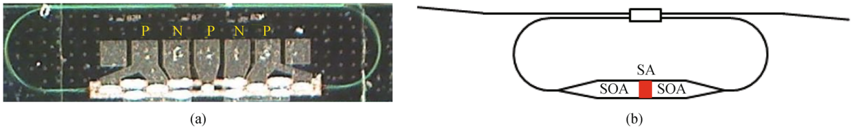
Fig. 6 (a) Photograph of the ring cavity colliding pulse mode-locked laser. The letters are added for clarity and denote the P and N contacts for the centered absorber and the two gain sections on either side; (b) schematic of the gain, absorber and waveguide sections inside the laser cavity. SA-saturable absorber, SOA-semiconductor optical amplifier
