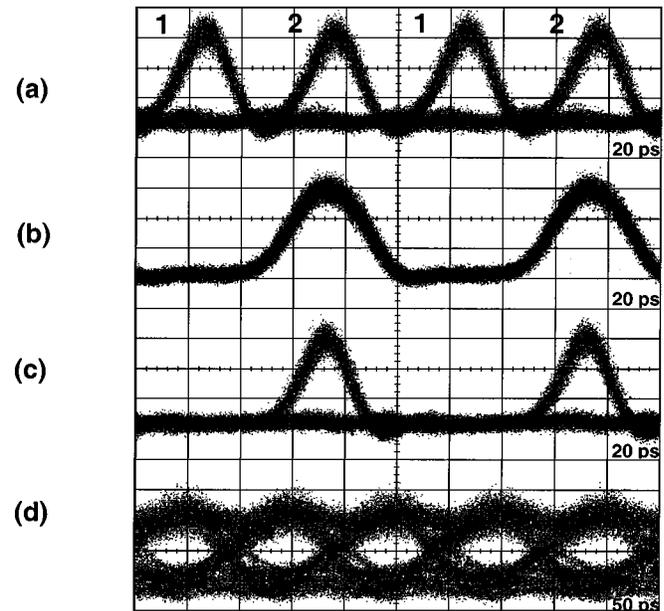
Fig. 3. Eye diagrams. (a) The 20-Gb/s OTDM data stream input to the EA modulator at port 1. (b) Optical transparency gating of the EA modulator aligned to channel 2. (c) The 10-Gb/s channel 2 transmitted in an optically transparent manner at port 3. (d) Simultaneously demultiplexed and O/E converted 10-Gb/s channel 1 at port 4.
