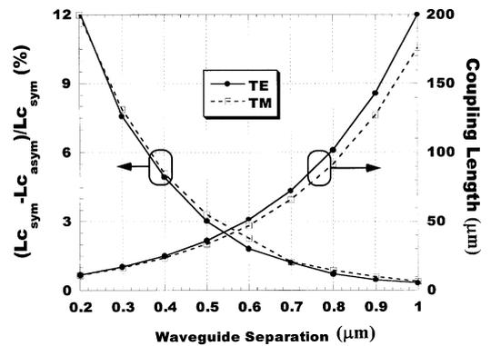
Fig. 5. Coupling length of the asymmetric coupler for the different values of  $n_a$  corresponding to Fig. 4 and its percent difference with respect to the symmetric case as a function of waveguide separation.
