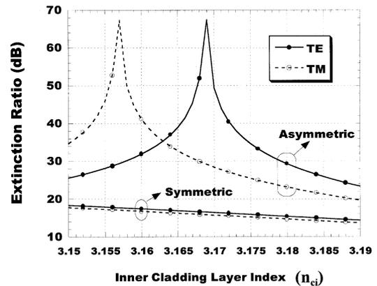
Fig. 7. Extinction ratio for TE and TM modes for the asymmetric and symmetric structures as a function of refractive index of inner cladding layer.
