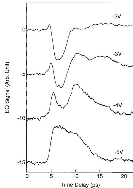
Fig. 3. Bias dependent responses with 68 fC photogenerated carriers in the intrinsic region. Data are vertically displaced for clarity.
