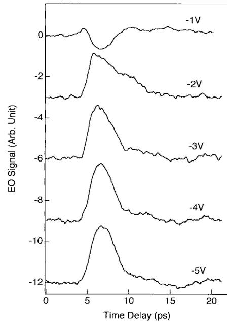
Fig. 2. Bias dependent responses with 29-fC photogenerated carriers in the intrinsic region. Data are vertically displaced for clarity.
