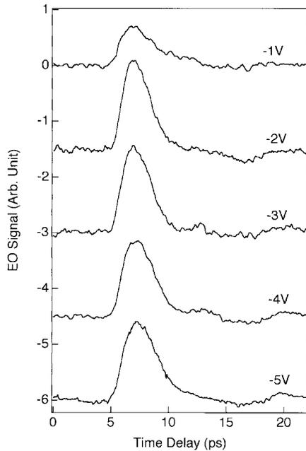
Fig. 1. Bias dependent responses with 13-fC photogenerated carriers in the intrinsic region. Data are vertically displaced for clarity.
