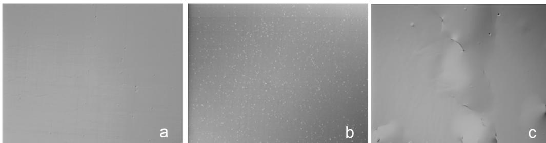
**Figure 4.13a-c** Nomarski micrographs of exposed surfaces after double bonding process. From left to right: good surface, high microscopic void density, large-scale cracking
