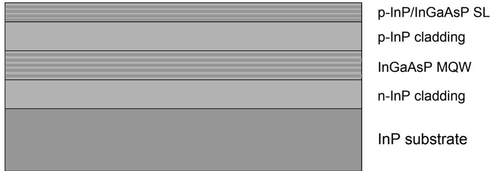
**Figure 3.8 InGaAsP/InP p-i-n active region with superlattice cap**
