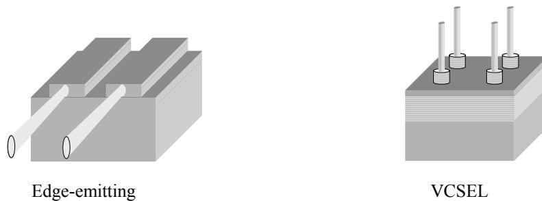
Figure 1.1 Schematic of edge-emitting and vertical cavity surface-emitting lasers
