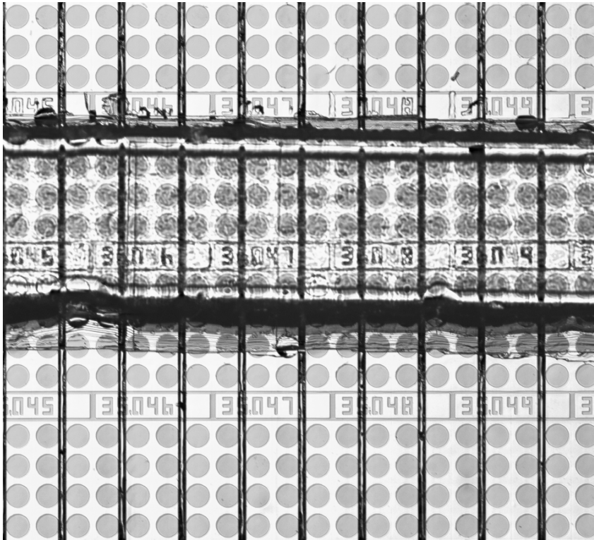
Figure 5.33. Photograph of completed CWDM VCSEL array. The material in the center is the etched bending accommodation region and the smooth areas on the top and bottom of the photo are the VCSEL regions.
