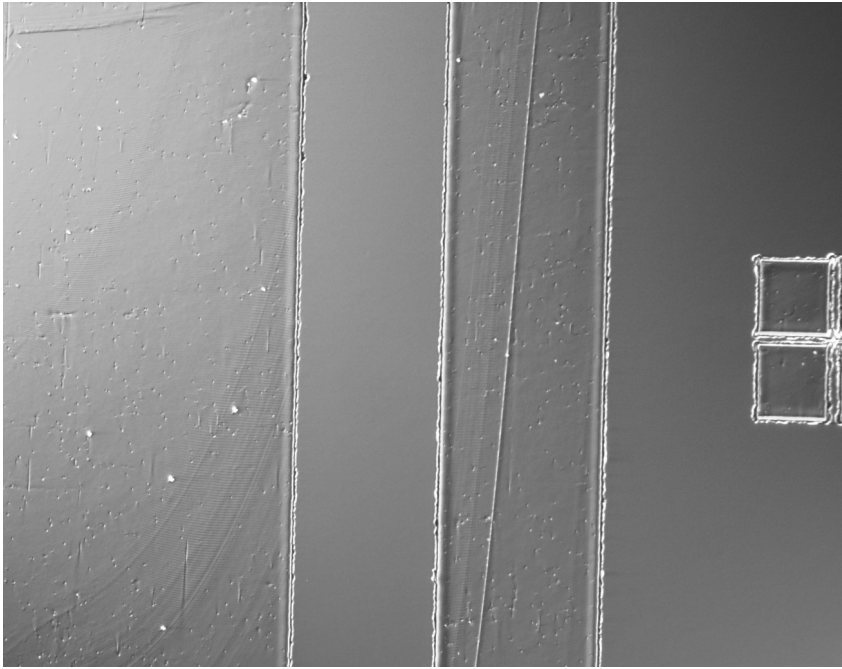
Figure 5.15. Photograph of a 3.75- \mu\text{m} deep etch with \text{H}_3\text{PO}_4:\text{HCl} (3:1) in ultrasound. The etch rate was 1.25 \mu\text{m} per minute. The area size shown is about a 2-mm square.
