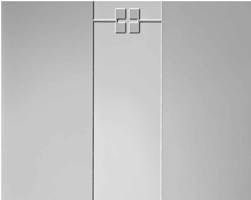
Figure 5.9. Photograph of small area of the sample surface after step etching. The center, raised region, is the top active region. The cross is an alignment target.
