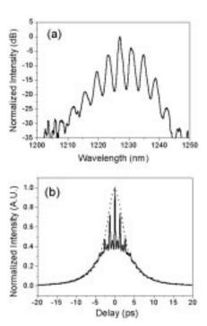
Fig. 7. (a) Output spectrum and (b) its corresponding autocorrelation trace of the multiwavelength Cr:forsterite laser output when the cover glass was turned 50° from normal incidence. Dotted line in (b) is a sech<sup>2</sup> fitting.
