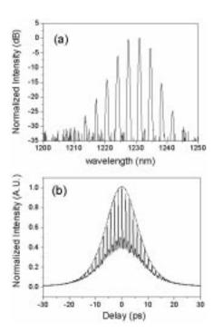
Fig. 6. (a) Output spectrum and (b) its corresponding autocorrelation trace of the multiwavelength Cr:forsterite laser output when the cover glass was turned 30° from normal incidence. Dotted line in (b) is a sech<sup>2</sup> fitting.
