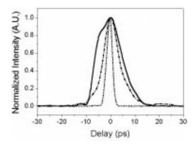
Fig. 5. Typical recovered channel pulse shape with  $0^{\circ}$  (solid curve),  $30^{\circ}$  (dashed-dotted curve), and  $50^{\circ}$  (dotted curve) incident angles of laser beam on the cover glass.
