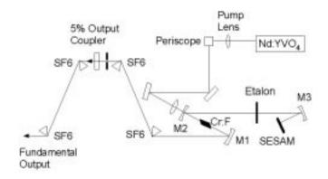
Fig. 1. Schematic diagram for the experimental setup.
