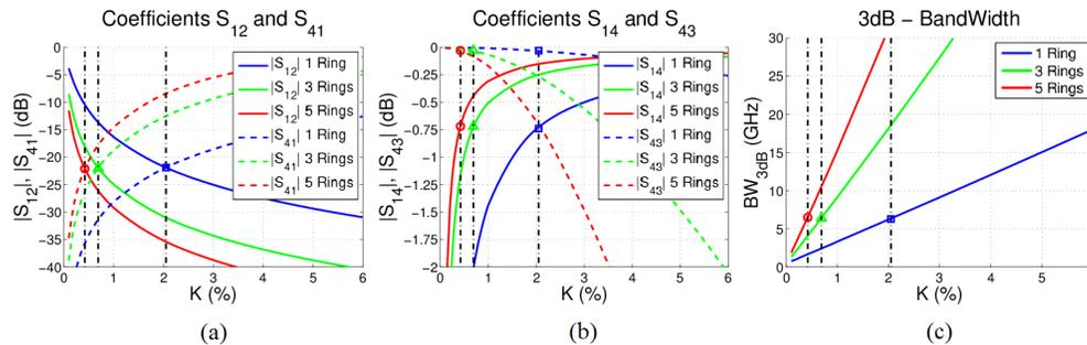
Fig. 7. Scattering coefficients at CW resonant frequency as a function of  $\kappa$  ( $a_{rr} = 1\text{ dB/cm}$ ) for  $R = 25\mu\text{m}$ .
