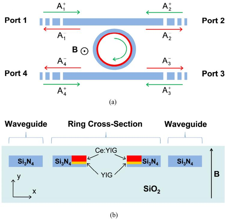
Fig. 1. Schematic structure of the TE-mode four-port optical circulator, Top view (a) and cross-section (b).
