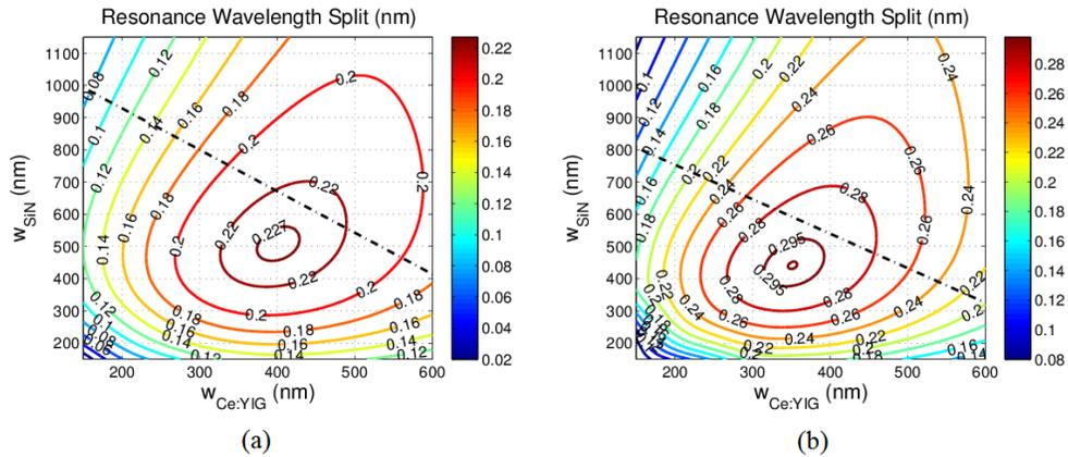
Fig. 3. Resonance wavelength split for the TE-circulator as a function of the silicon nitride ( $w_{\text{SiN}}$ ) and the magneto-optical material width ( $w_{\text{Ce:YIG}}$ ). Figures 3(a) and 3(b) refer to a 300nm and 400nm thick waveguide, respectively.
