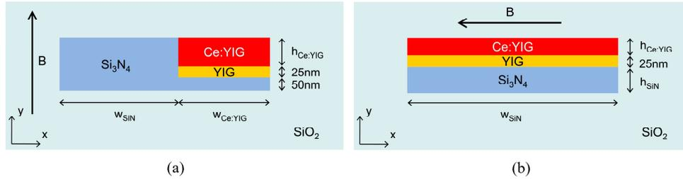
Fig. 2. Ring-cross section and external magnetic field direction for the TE-mode circulator (a) and TM-mode circulator (b).
