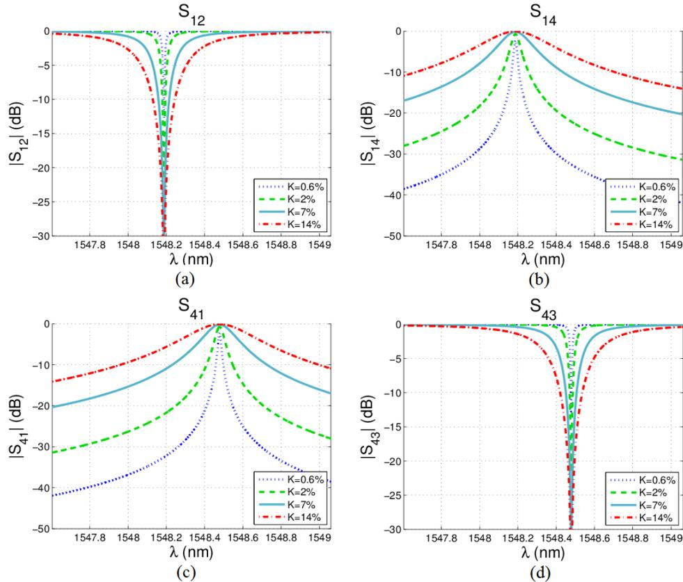
Fig. 6. Scattering coefficients as a function of wavelength  $\lambda$  and power coupling coefficients  $\kappa$ .
