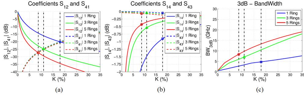
Fig. 8. Scattering coefficients at CW resonant frequency as a function of  $\kappa$  ( $\alpha_{rr} = 1\text{dB/cm}$ ) for  $R = 300\mu\text{m}$ .
