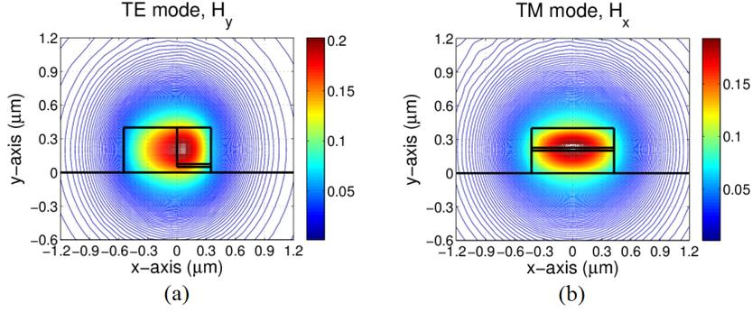
Fig. 5. Magnetic field profile of the principal component for TE-mode (a) and TM-mode (b) in the two circulators, respectively.
