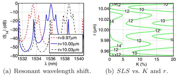
Fig. 6. Radius inaccuracy analysis. (a) Spectra of  $S_{14}(\lambda)$  for different  $r$  and  $K = 10\%$ . (b) Radius inaccuracy and  $K$  variation effects on SLS (dB).
