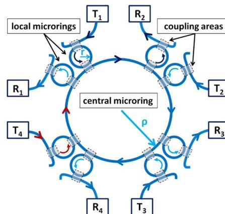
Fig. 1. MMR NoC architecture.
