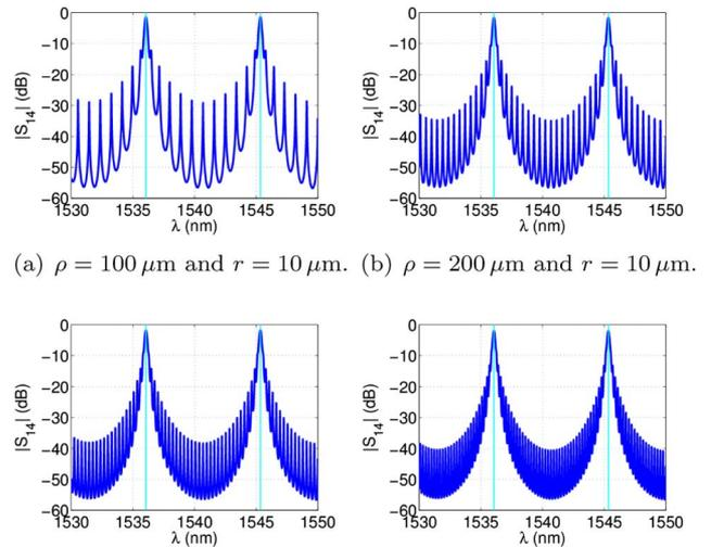
Fig. 5. Spectra of  $S_{14}(\lambda)$  for increasing values of  $\rho$ .
