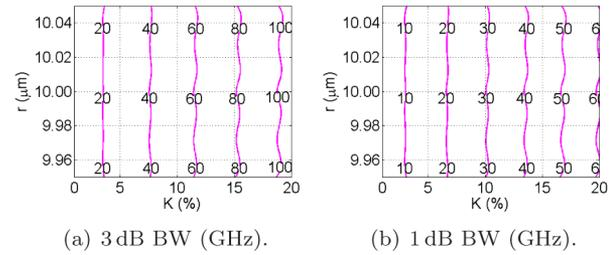
Fig. 7. Radius inaccuracy analysis. (a) 3 dB BW and (b) 1 dB BW with respect to  $K$  and  $r$ .
