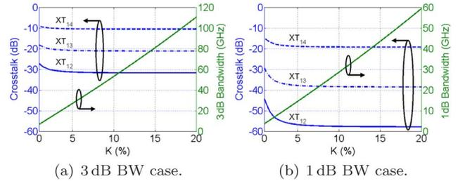
Fig. 4. BW and corresponding crosstalk with respect to  $K$  for  $r = 10 \mu\text{m}$  and  $\rho = 40 \mu\text{m}$ .
