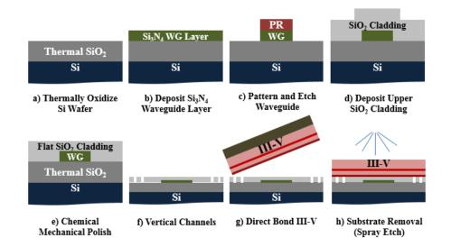
Figure 4.5: Simplified process flow diagram from bulk Si oxidation through bonding and substrate removal.
