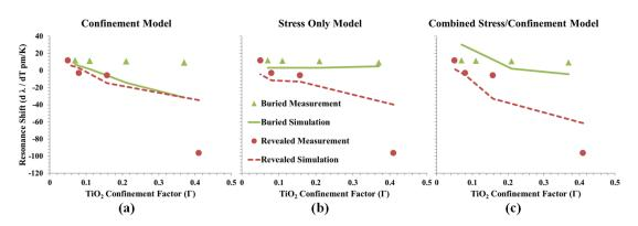
Figure 2.6: Comparison of the *confinement*, *stress*, and *combined stress/confinement model*.
