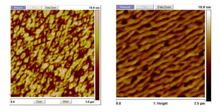
Figure 4.3: AFM scans of SL surface before bonding; (a) initial growth with InGaP SL (2.8 nm RMS) resulted in unsuccessful bonding; (b) second growth substituting the InGaP SL with InGaAs/GaAsP (1.1 nm RMS) resulted in successful bonding.
