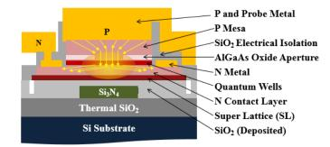
Figure 3.2: Laser cross-section. In bulk of the gain region, mode is entirely in III-V so Si3N4 waveguide width reduces to zero over the course of the tapered mode converter and the mode is guided by the  $AlO_x$  aperture
