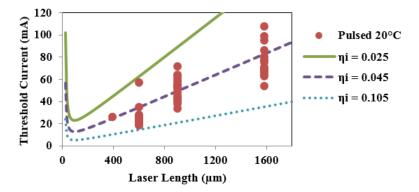
Figure 3.6: 20°C pulsed threshold current data for 12  $\mu m$  mesas with 4  $\mu m$  wide current apertures 300°C O<sub>2</sub> plasma assisted bonded to 5  $\mu m$  of SiO<sub>2</sub> on Si.
