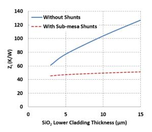
Figure 3.21: Comparison of thermal impedance  $Z_t$  v. SiO<sub>2</sub> lower cladding thickness for unshunted and shunted lasers. Two 5  $\mu m$  wide Au shunts are placed on either side of the 20  $\mu m$  mesa. There is a 200 nm buffer of SiO<sub>2</sub> between the shunt and the bonding interface.
