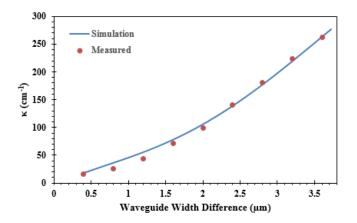
Figure 3.15: Measured and simulated grating strength for 1000  $\mu m$  long gratings under TE excitation. The widest waveguide width is always 2.8  $\mu m$ . The plot also gives fitted and simulated coupling constant values for the same set of gratings.
