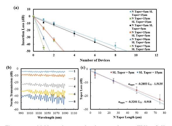
**Figure 3.10:** (a) Measured insertion loss for repeated passive III-V to  $Si_3N_4$  tapers plotted by number of serial repeats of a single device. (b) Normalized transmission spectra for (1, 2, 4, 6 & 8) repeats of lowest loss taper. (c) Taper loss is plotted from the repeated taper data in (a) after removing bulk loss.
