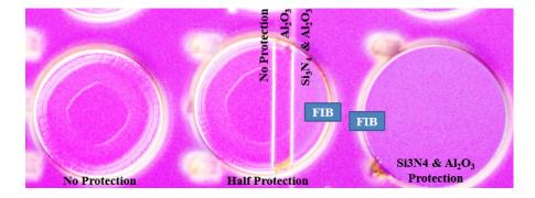
Figure 4.12: Nomarski mode image of round test structure mesas including one with no protection, one with half protection and one that is fully protected of 90 nm PECVD silicon nitride and 30 nm ALD Al<sub>2</sub>O<sub>3</sub>
