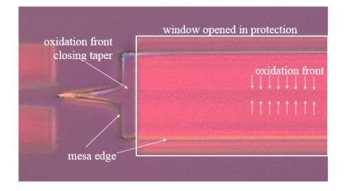
Figure 4.11: Example of selective area oxidation of a wide mesa device with unwanted oxidation observed in the tapered section which is covered with a protection dielectric.
