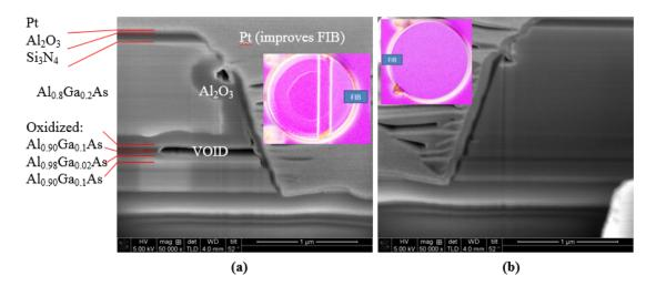
Figure 4.13: Comparison of FIB cross sections in adjacent mesas labeled in Fig. 4.12 and placed in the inset of each SEM image. (a) Shows oxidized area of protected feature of mesa and a 1  $\mu m$  void at the oxidation layer. (b) Shows an entirely protected mesa with no signs of oxidation at all and no void.
