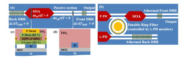
**Figure 2.13:** (a) Passively Athermal DBR Laser (b) Athermal Ring Filtered DBR (ARF-DBR) Laser (c) cross section of III-V/Si Hybrid SOA or PD with TiO<sub>2</sub> cladding. (d) cross section of Si waveguide clad with TiO<sub>2</sub> for a thermal compensator.
