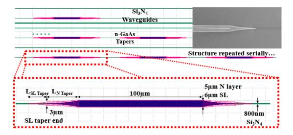
Figure 3.9: Layout of repeated taper structures with labels on key geometries. Mask splits included length of SL taper, and length of N Taper. Taper tips  $\sim 200$  nm. Structures do not include active quantum well mesa.
