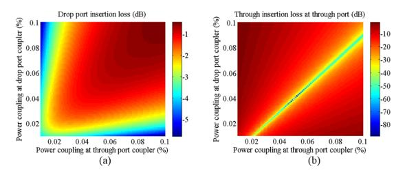
Figure 2.15: (a) Drop port insertion loss in dB of a ring filter (i.e. from the SOA to the rear mirror in Fig. 2.13(a). (b) Through port insertion loss in dB (i.e. from the SOA to the P-PD in Fig 2.13(a). Assumes 1dB/cm propagation loss, 25  $\mu m$  ring radius.
