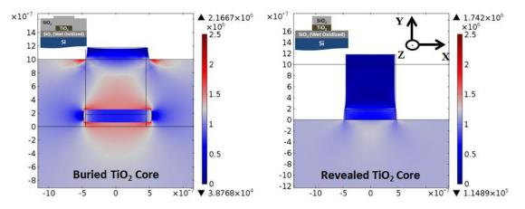
Figure 2.7: Comparison of the thermal stress profile of buried and revealed core waveguides.
