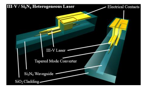
Figure 3.1: Schematic of III-V/Si<sub>3</sub>N<sub>4</sub> heterogeneous laser directly coupled via III-V tapers through the III-V/SiO<sub>2</sub> cladding bonding interface. (artwork courtesy of Martijn Heck)
