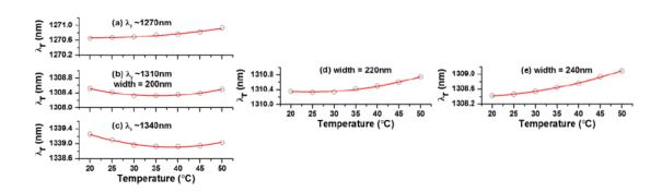
**Figure 2.11:** Measured (black circle) and quadratically fitted (red line) resonance wavelength as a function of temperature. The device with a waveguide width of 200 nm is measured at various spectral ranges around (a) 1270 nm, (b) 1310 nm and (c) 1340 nm and across different waveguide widths (b) 200 nm, (d) 220 nm, (e) 240 nm [74].
