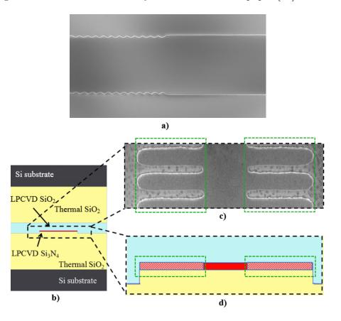
**Figure 3.12:** (a) SEM image of sidewall DBR in LPCVD  $Si_3N_4$  strip with subtle perturbation. (b) Waveguide cross-section for C-band ultra-low loss waveguide. (c) SEM image of strong perturbation for reference to (d) a zoomed in cross-section with shaded grating areas.
