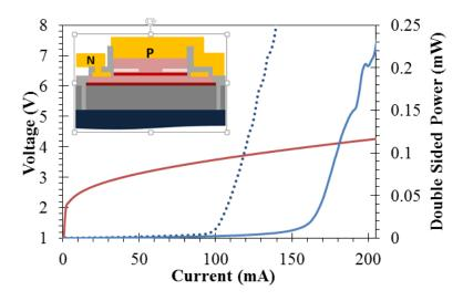
**Figure 3.4:** CW (red) IV and (blue) LI curves of a 2400  $\mu m$  long Fabry-Pérot laser. Inset shows a cross-sectional schematic.
