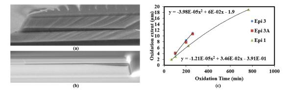
**Figure 4.10:** (a) SEM image of bonded (cladding on top) mesa oxidation profile from Epi 1. (b) SEM image of unbonded (cladding on bottom) test mesa oxidation profile from Epi 3. (c) Measured AlGaAs oxidation extents over a range of times for 3 epi with two different aperture layer designs.
