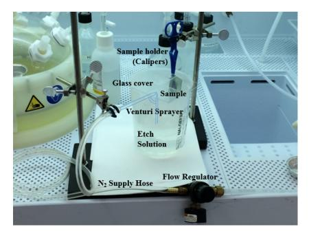
Figure 4.2: Photograph of spray etch setup as adapted from the setup in [96].
