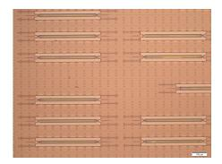
Figure 4.7: Selective placement of vertical channels was made to prevent them from expanding into bubbles and possibly exploding during high-temperature oxidation or contact anneal processes.
