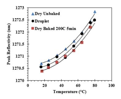
Figure 2.9: Peak reflectivity of 200 nm wide, 200 nm height third order DBR gratings as a function of temperature. Sample was tested following cleaning and  $N_2$  drying, first without baking (typical), second with a water droplet on top (high humidity), and finally after a 5 min 200°C dehydration bake (low humidity) [74].
