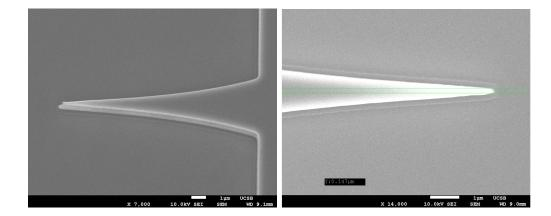
Figure 4.19: Characteristic p-mesa tapers following  $Cl_2/N_2$  dry etch with SiO<sub>2</sub> hardmask and  $H_2SO_4:H_2O_2:H_2O$  (1:1:10) wet etch. (right) measurement of hardmask taper tip width is 147 nm.
