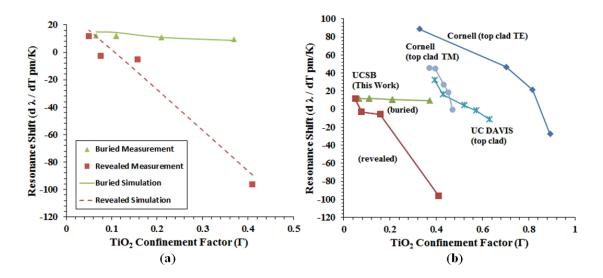
**Figure 2.5:** (a) Measured thermal drift with *confinement models* based on Eq. 2.9 with separately fitted  $\text{TiO}_2$  TOC for buried  $(-10^{-6}K^{-1})$  and revealed  $(-2.5 \times 10^{-4}K^{-1})$  rings. (b) Measurements compared to other literature with  $\text{TiO}_2$  cladding demonstrate a unique suppression of TOC in buried  $\text{TiO}_2$ .
