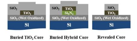
Figure 2.4: Cross section of waveguide designs with TiO<sub>2</sub> or hybrid cores.
