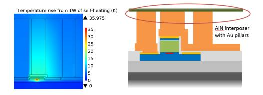
Figure 3.22: Thermal simulation showing the release of thermal energy primarily out of the mesa. Mesa is 20  $\mu m$  wide with 1.520  $\mu m$  tall mesa and made of Al<sub>0.8</sub>Ga<sub>0.2</sub>As.
