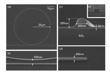
Figure 2.10: (a) Top-view SEM image of ring resonator before TiO2 cladding deposition; (b) Ring-to-bus waveguide coupling region; (c) Cross-sectional SEM image of waveguide before TiO2 cladding deposition; (d) Top-view SEM image of inverse taper. (e) Shows the waveguide following TiO<sub>2</sub> cladding with small voids in the deposited film [74].
