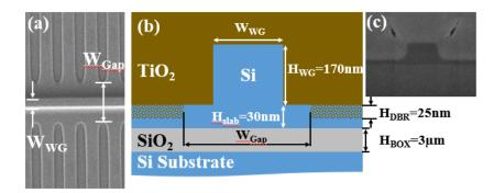
Figure 2.8: Waveguide geometries. (a) top down SEM image of DBR before TiO2 top cladding deposition, (b) cross-sectional diagram of DBR. (c) Cross-sectional SEM of TiO<sub>2</sub> clad Si waveguide with small voids visible in the TiO<sub>2</sub> [74].
