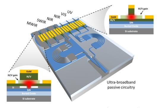
Figure 5.1: Schematic of a fully-integrated UV-MIR (6-bands shown) single-chip emitter concept, showing the two regions of the wafer with Si-on-Si<sub>3</sub>N<sub>4</sub>-on-SiO<sub>2</sub>-on-Si and more standard Si and Si<sub>3</sub>N<sub>4</sub> waveguides. (Artwork courtesy of Martijn Heck.)
