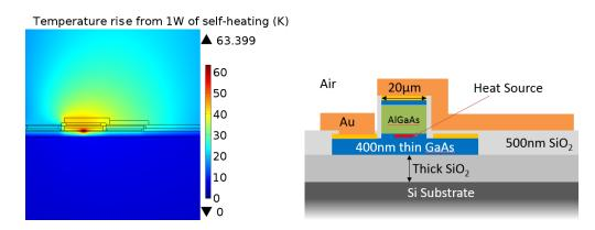
Figure 3.16: 5  $\mu m$  wide Au shunts positioned directly under the sides of a 20  $\mu m$  mesa result in a thermal impedance of 63.4 K/W.
