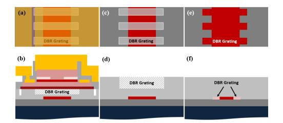
**Figure 3.11:** (a-b) Top and cross-section of surface corrugated gratings underneath bonded III-V lasers (c-d) Top and cross-section of surface corrugated gratings into top cladding of passive waveguide. (e-f) Top and cross-section of sidewall passive gratings.
