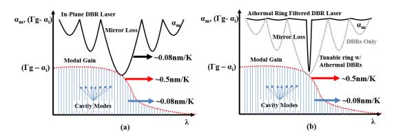
Figure 2.12: (a) Diagram of typical in-plane semiconductor laser with dense cavity modes where thermal drift is typically dominated by cavity loss. (b) A similar DBR laser design with and intra-cavity ring filter to achieve a narrower reflectivity bandwidth.
