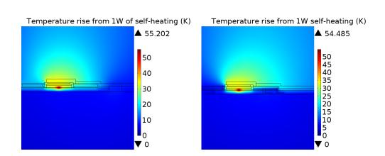
Figure 3.18: Comparison of probe and n-metal shunts. N-metal shunts 1.5  $\mu m$  wide were added 25  $\mu m$  from the center of the 20  $\mu m$  mesa. A single 10  $\mu m$  wide probe shunt is added to the 2  $\mu m$  thick p-probe and shunted 40  $\mu m$  from the mesa.
