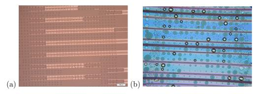
**Figure 4.6:** (a)Microscope image of the original placement of VCs under thin n-contact material. (b) Microscope image following a high-temperature process with a full thin n-layer. Most VCs burst and redeposited material onto the sample.
