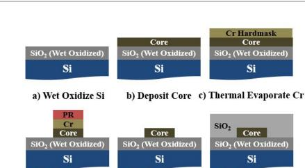
d) Lithography & Dry e) Dry Etch Mask f) SiO<sub>2</sub> Covering Etch Mask & Core (optional)
