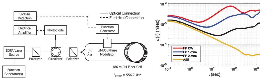
Fig. 1. (left) Schematic of in-house assembled fiber-based optical gyroscope. All fibers after the first polarizer are PM and input polarization is optimized for maximum power at the photodiode. Components are connected with FC/APC connectors. (right) Allan deviation measurements for an FP laser at CW, single, and two-tone modulation compared to an ASE source.
