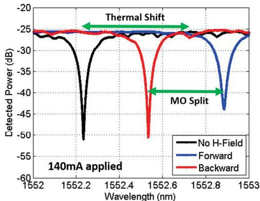
**Fig. 4:** Experimental results showing both the nonreciprocal MO wavelength split as well as the thermally induced redshift.
