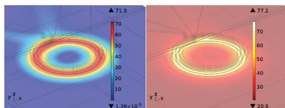
Fig. 2: Multiphysics simulation results: a) radial magnetic field generated by the electric current  $I=180\text{ mA}$ , b) temperature distribution in the device
