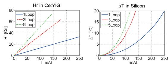
Fig. 3: Electromagnet comparison a) radial magnetic field at the silicon-Ce:YIG interface b) average temperature variation in the silicon ring
