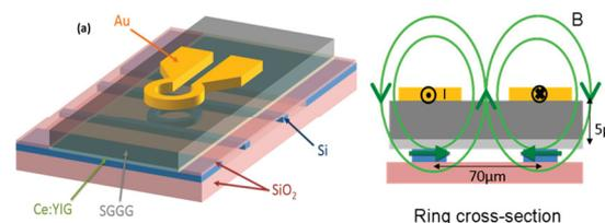
**Fig. 1:** (a) Perspective view and (b) cross-sectional view of a proposed optical circulator with integrated electromagnet.
