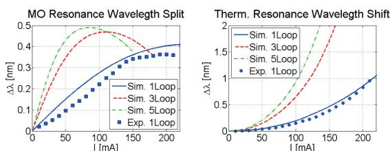
**Fig. 5:** Electromagnet comparison a) MO resonance wavelength split b) thermal resonance wavelength shift
