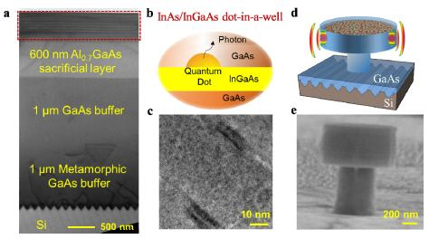
A schematic illustration of the epitaxial layers and QDs active region are shown in Fig. 1(a) and Fig. 1(b) respectively. A high resolution transmission electron microscope (TEM) image in Fig. 1(c) reveals the typical dot size, which has a diameter of  $\sim$ 21 nm and height of  $\sim$ 6 nm. By combing the colloidal lithography, dry-etching and subsequent wet-
