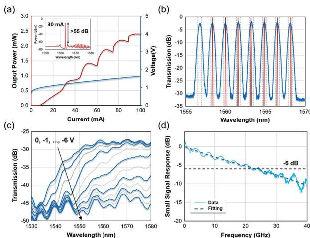
**Fig. 3.** (a) LIV curve and spectrum of integrated DFB, (b) transmission spectrum of cascaded AWGs with aligned DFB spectrum with normalized power level, (c) transmission spectrum of EAM at various biases, and (d) small signal response of a Tx-Rx channel.
