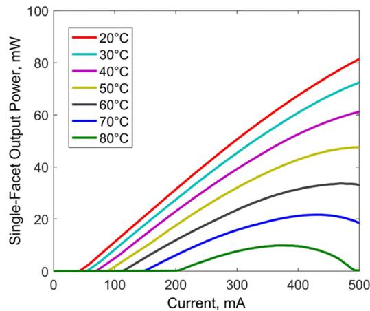
Fig. 7. Continuous wave light output power as a function of injection current for a  $8 \times 1200 \mu\text{m}^2$  device with one polished facet and one 95% high reflection coated facet at temperatures from 20 to 80°C.
