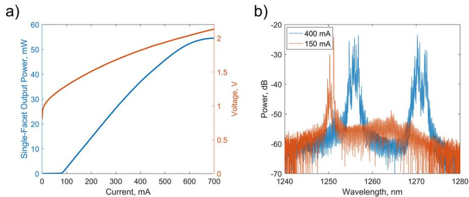
Fig. 5. (a) Continuous wave light output and voltage as a function of the injection current of a  $9 \times 1200 \mu\text{m}^2$  device showing a threshold of 81 mA and maximum single-side output power of 55 mW. (b) The above threshold optical spectrum showing ground state lasing near 1250 nm which transitions to dual lasing attributed to multimode lasing from higher order transverse modes. Excited state lasing was not observed for the given injection levels.
