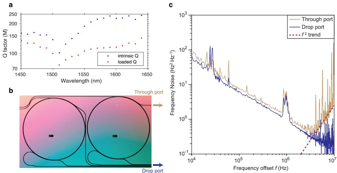
**Fig. 1:** (a) Intrinsic and loaded  $Q$  factors of a ring resonator featuring a drop port, measured at various wavelengths. (b) Optical micrograph of the fabricated ring resonator with 10.8 GHz FSR. (c) Frequency noise of the DFB laser operating at 1556 nm when self-injection-locked to the resonator, measured from the through port and drop port.
